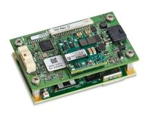
The new SPAN supported MEMS sensors are coupled with NovAtel's SPAN receivers using a new compact, lightweight MEMS Interface Card (MIC) designed to support both power and communication. The MIC is NovAtel's smallest receiver form factor, providing integrators an extremely compact, powerful GPS/INS engine. Designed as a board stack configuration for ease of integration, the interface card can be directly interfaced to NovAtel's small OEMV-1DF SPAN receiver.
